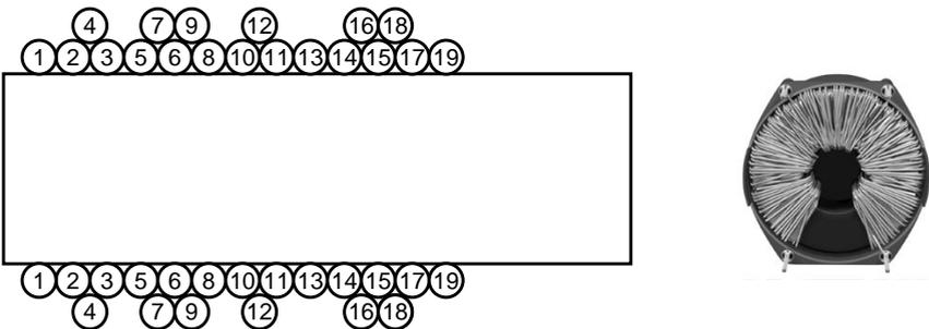
The winding pitch is smaller than the wire diameter. The coil is wound in one direction only. This method of winding a coil does not permit the final position of a turn to be predetermined exactly. The cross section of this type of winding clearly shows a disorderly, "random" arrangement of the turns. This leads to the parasitic capacitances being only minimally greater than those achieved by single-layer winding, and the resonance frequencies are equal to those achieved by single-layer winding.
