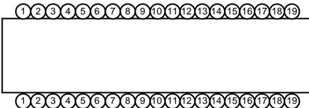
The winding pitch is equal to or greater than the wire diameter. The coil is wound in one direction only. The only capacitances (parasitic capacitances) are those between one turn to the next. In comparison to all other types of winding, this type of winding leads to the lowest possible capacitances and thus the highest resonance frequencies.
