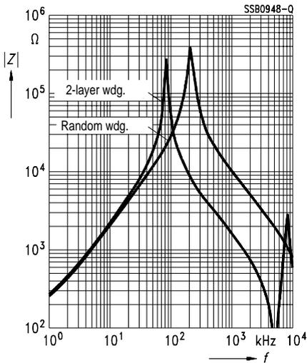
Fig. 13 Impedance  $|Z|$  versus frequency  $f$
