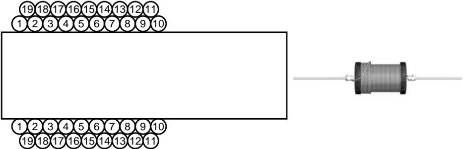
The winding pitch is equal to the wire diameter. The coil is wound with several layers. This leads to parasitic capacitances between the layers in addition to the turn-to-turn capacitances. In comparison to all other types of winding, this type leads to the highest capacitances and thus the lowest resonance frequencies.
