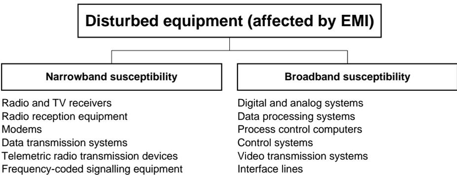
Fig. 6 Disturbed equipment
