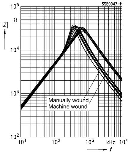
Fig. 14 Impedance  $|Z|$  versus frequency  $f$
