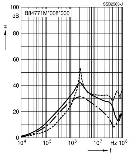
**Insertion loss for medical versions (typical values at  $Z = 50 \Omega$ )**
