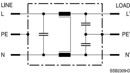
**Typical circuit diagram of B84771M\*
