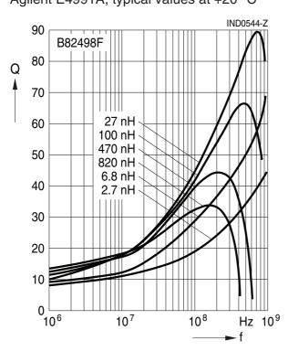
Q factor versus frequency f (ferrite core) measured with impedance analyzer Agilent E4991A, typical values at +20 °C
