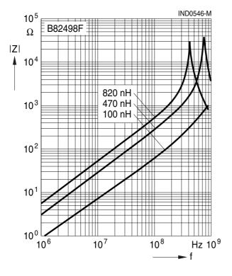
Impedance IZI vs. frequency f (ferrite core) measured with impedance analyzer
