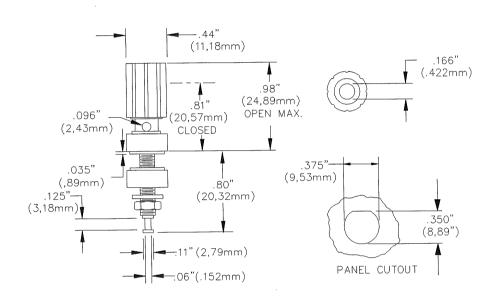
Mounts in Panels between .070" and .250" (1.77-6.35) Thick Accepts Standard 4mm Banana plugs or bare wire or spade lugs
