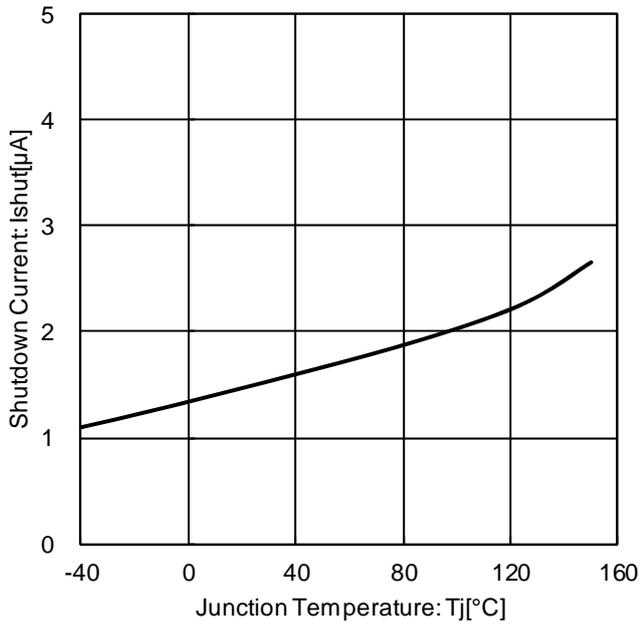
Figure 21. Shut Down Current vs. Temperature (CTL = 0 V)
