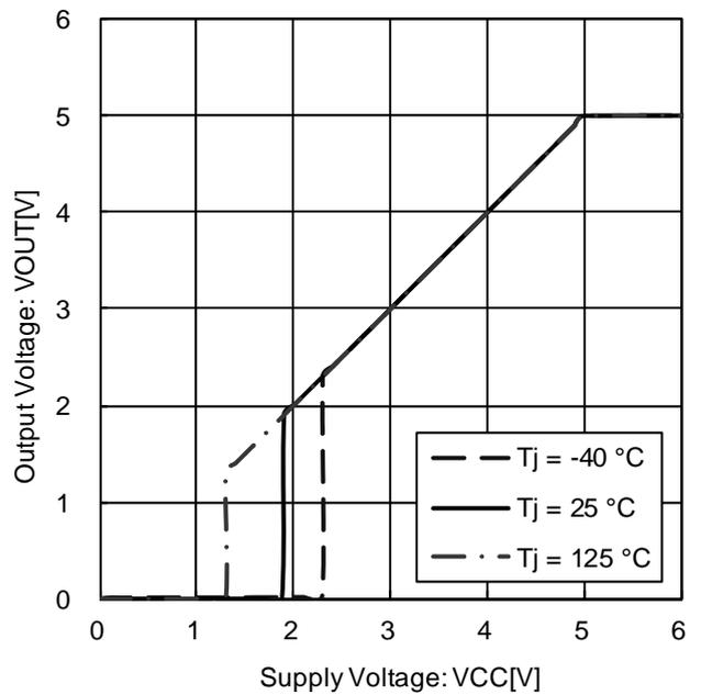
Figure 26. Output Voltage vs. Power Supply Voltage ( $I_{OUT} = 0\text{ mA}$ )
