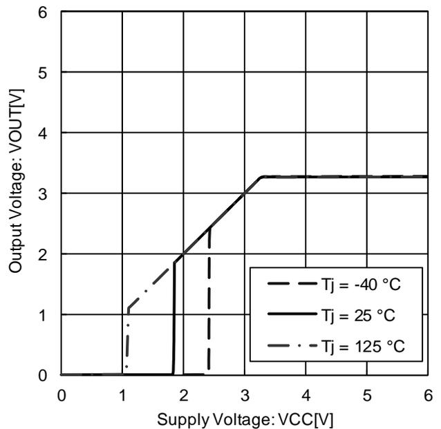
Figure 8. Output Voltage vs. Power Supply Voltage ( $I_{OUT} = 0\text{ mA}$ )
