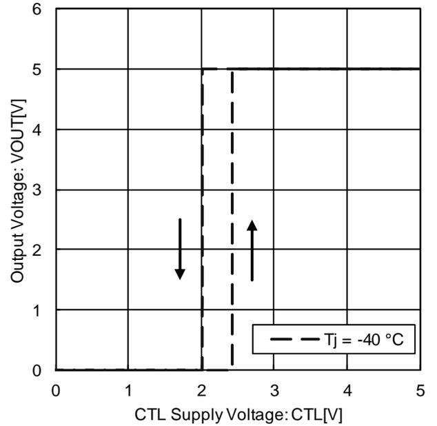
Figure 36. CTL ON / OFF Mode Voltage ( $T_j = -40\text{ }^{\circ}\text{C}$ )
