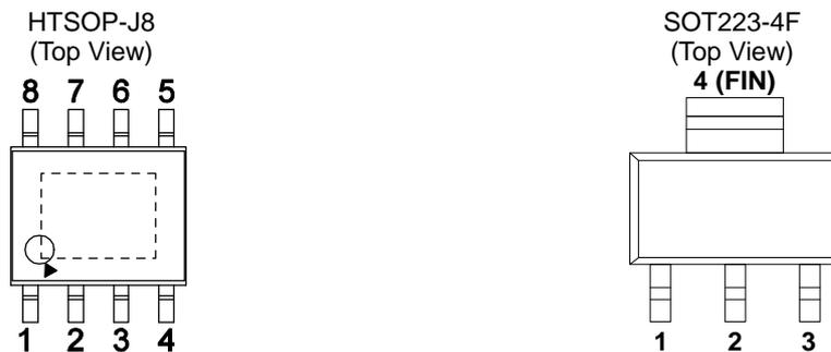
Figure 3. Pin Configuration
