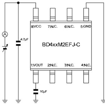
Measurement Setup for Figure 5, 7, 16, Figure 23, 25, 34
