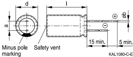
Safety vent for diameter  $\geq 8$  mm.
