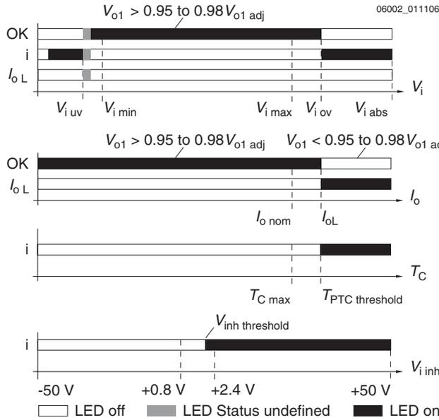
LEDs "OK", "i" and "IoL" status versus input voltage
