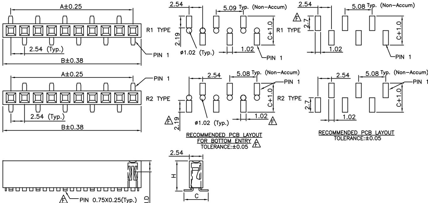
Height=5.0mm: Min. Insertion Depth = 1.55mm
