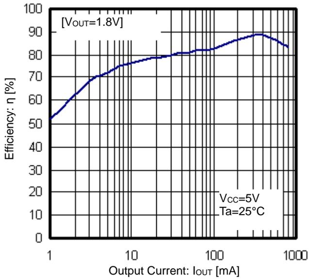
Figure 14. Efficiency vs Output Current
