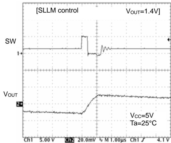
Figure 66. SW Waveform (Io=10mA)
