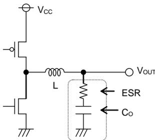
Figure 97. Output Capacitor
