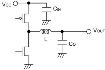
Figure 98. Input Capacitor
