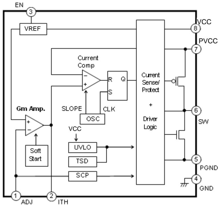
Figure 9. BD9120HFN Block Diagram
