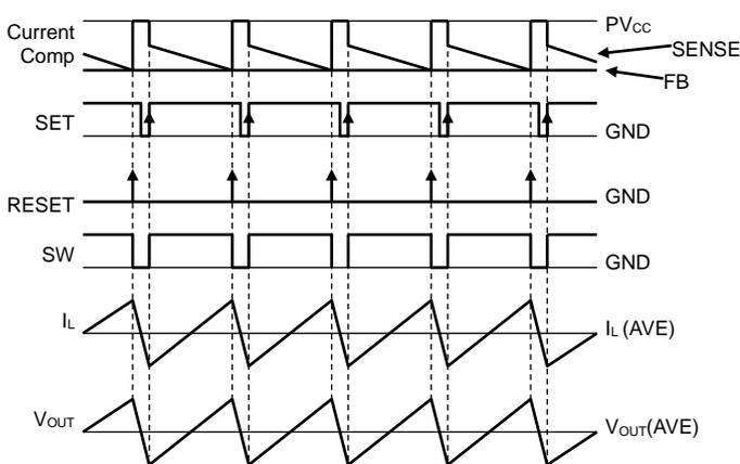
Figure 86. PWM Switching Timing Chart
