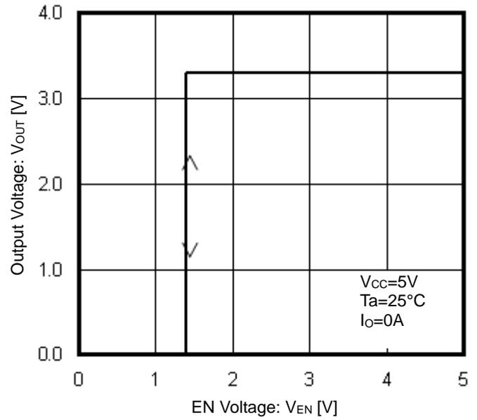
Figure 41. Output Voltage vs EN Voltage
