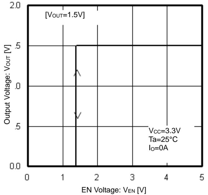
Figure 71. Output Voltage vs EN Voltage
