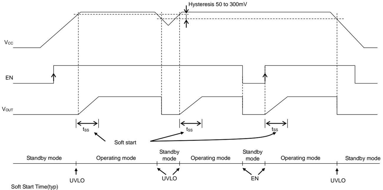
Figure 88. Soft Start, Shutdown, UVLO Timing Chart
