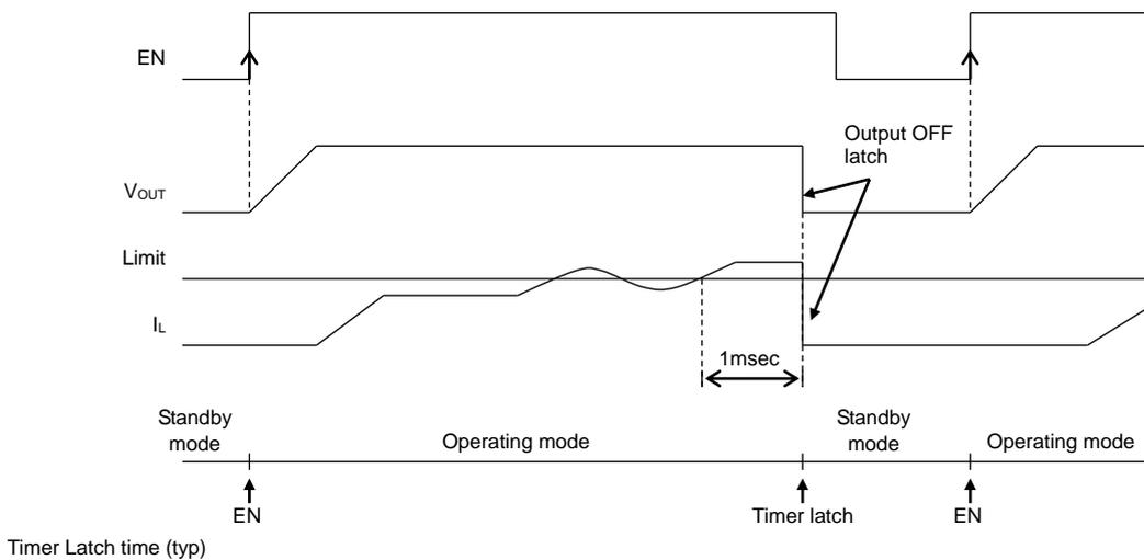
Figure 89. Short-circuit Protection with Time Delay Diagram
