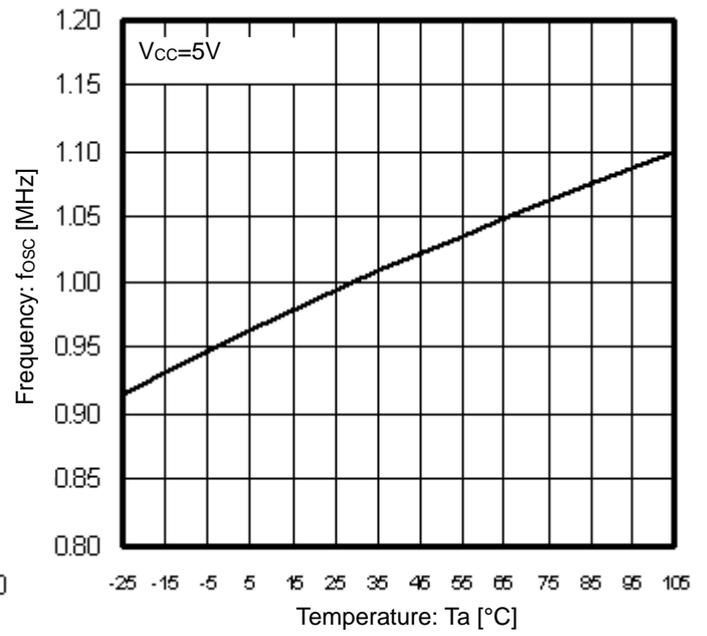
Figure 60. Frequency vs Temperature
