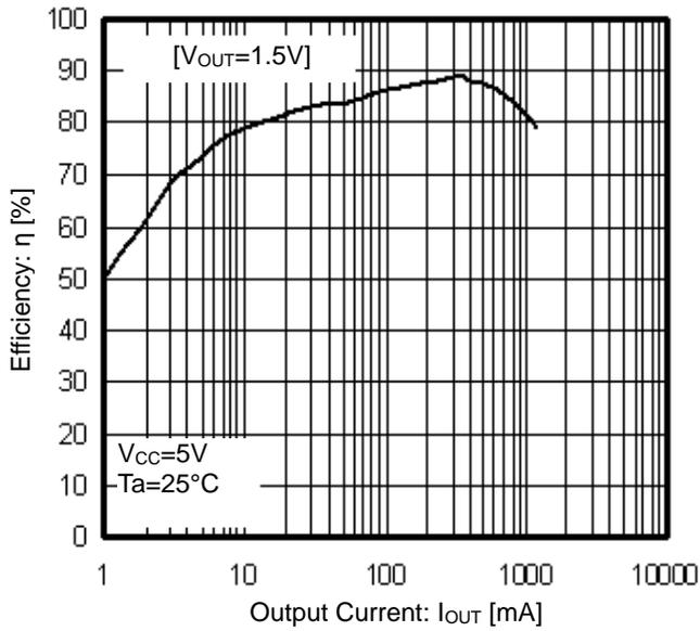
Figure 29. Efficiency vs Output Current
