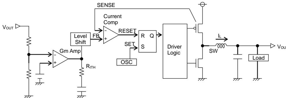
Figure 85. Diagram of Current Mode PWM Control
