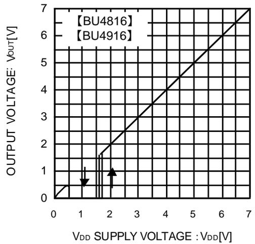
Fig.6 I/O Characteristics
