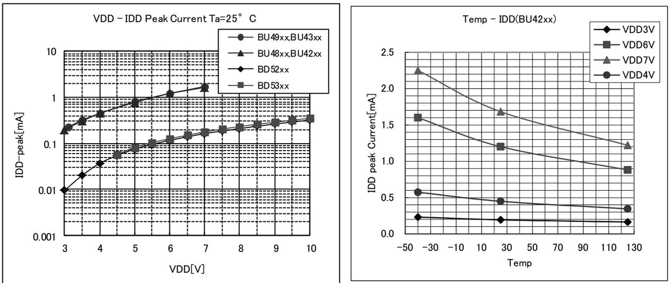
Fig.19 Current Consumption vs. Power Supply Voltage
