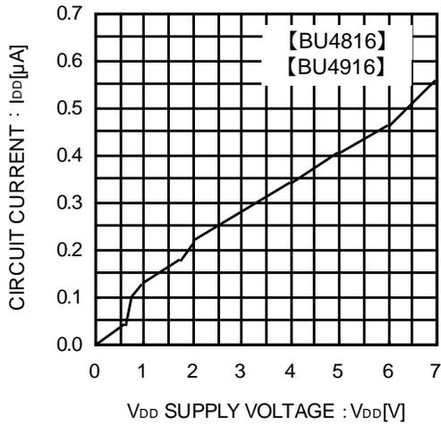
Fig.3 Circuit Current
