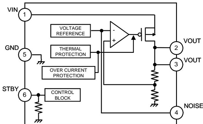
Figure 2. Block diagram
