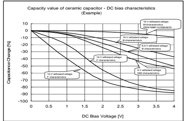
Figure 11. Capacity-bias characteristics
