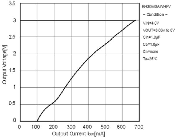
Figure 5. Output Voltage vs. Output Current (OCP Threshold)
