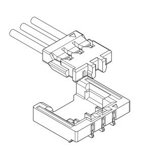
This ACHF connector is compact and low profile type, height 1.43mm and width 4.95mm, 1.2mm pitch wire-to-board connector. • High-strength
