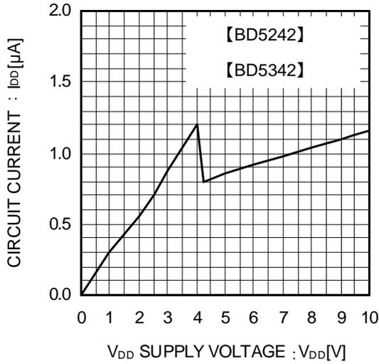
Fig.3 Circuit Current
