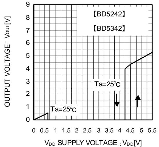
Fig.6 I/O Characteristics
