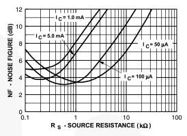
Figure 8. Noise Figure vs. Source Resistance
