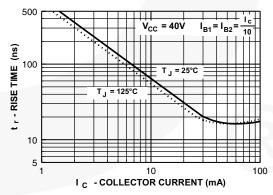
Figure 12. Rise Time vs. Collector Current
