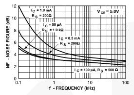
Figure 7. Noise Figure vs. Frequency
