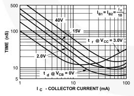
Figure 11. Turn-On Time vs. Collector Current
