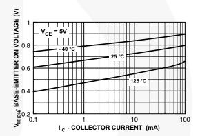
Figure 4. Base-Emitter On Voltage vs. Collector Current
