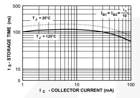
Figure 13. Storage Time vs. Collector Current
