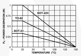
Figure 10. Power Dissipation vs. Ambient Temperature
