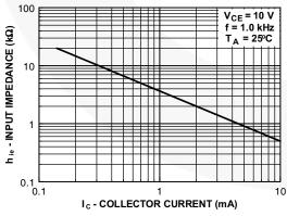
Figure 17. Input Impedance
