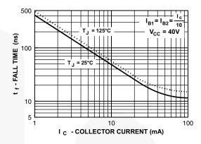
Figure 14. Fall Time vs. Collector Current
