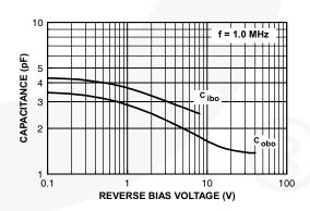
Figure 6. Capacitance vs. Reverse Bias Voltage
