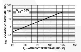
Figure 5. Collector Cut-Off Current vs.
