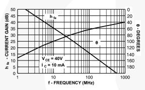
Figure 9. Current Gain and Phase Angle vs. Frequency
