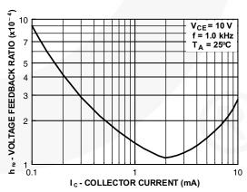
Figure 18. Voltage Feedback Ratio
