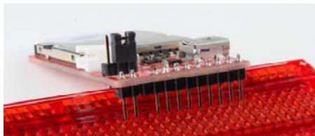
*Pins soldered onto the imp Breakout Board*
