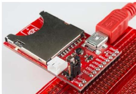
*In this image, the jumper is set to apply USB power to the imp breakout. A JST connector was soldered to the battery input pins, in case we want to use a LiPo to power the board.*
