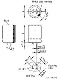
Snap-in capacitors are also available with 3 terminals (length (4.5 – 1) mm). PET insulation is marked with label "PET" on the sleeve. Safety vent on the case wall.
