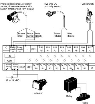
Note: IEC wire colors for photoelectric sensors and proximity sensors are shown first. The colors in parentheses refer to the old colors.
