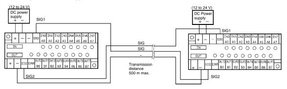
Note: A twisted pair or VCTF cable with a thickness of 0.75 mm<sup>2</sup> min. must be used for signal transmission.
