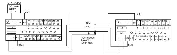
Note: In this example, a twisted pair or VCTF transmission cable with a thickness of 0.75 mm<sup>2</sup> min. is used, through which a current of 1.8 A max. can be transmitted.
