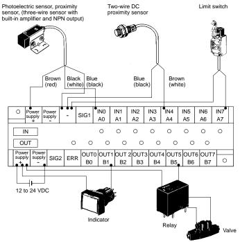
Note: IEC wire colors for photoelectric sensors and proximity sensors are shown first. The colors in parentheses refer to the old colors.
