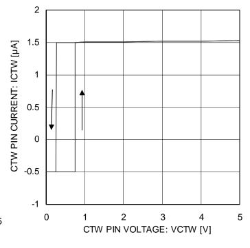
Figure 6. CTW Charge Discharge Current
