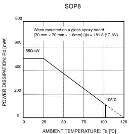
Figure 16. Power Dissipation
