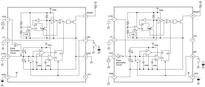
CT pin capacitor: 470pF to 3.3µF CTW pin capacitor: 0.001µF to 10µF
