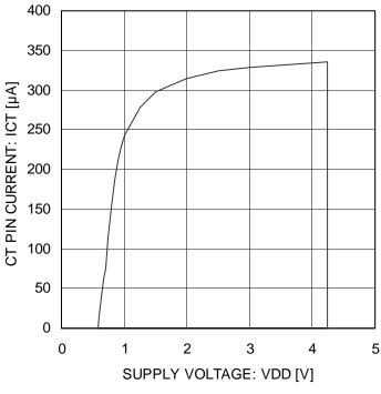
Figure 5. Delay Pin Current vs Power Supply Voltage
