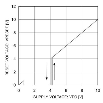
Figure 3. Detection Voltage
