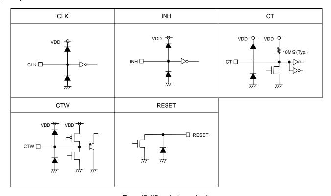
Figure 17. I/O equivalence circuit
