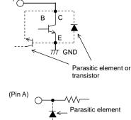
Figure 18. Example of IC structure
