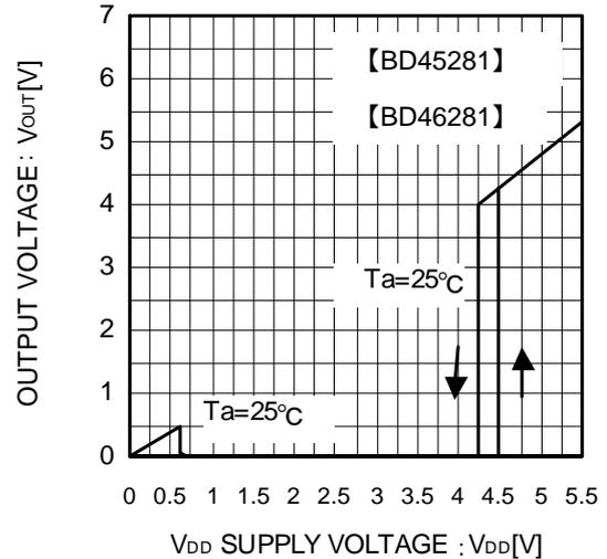
Fig.6 I/O Characteristics
