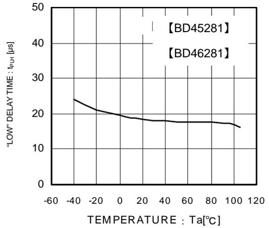
Fig.14 Output Delay Time
