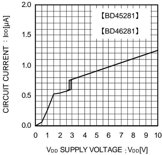
Fig.3 Circuit Current
