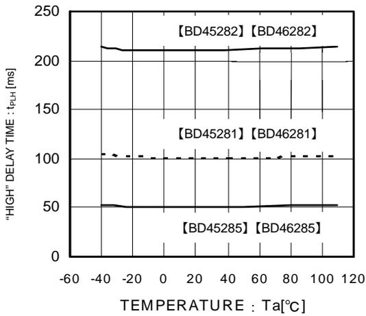
Fig.13 Output Delay Time
