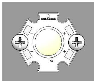
Figure 42: Recommended Mounting Locations for Hexagonal Star Products
