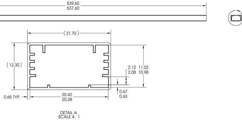
Figure 47: Tube Design for Rectangular Array Products
