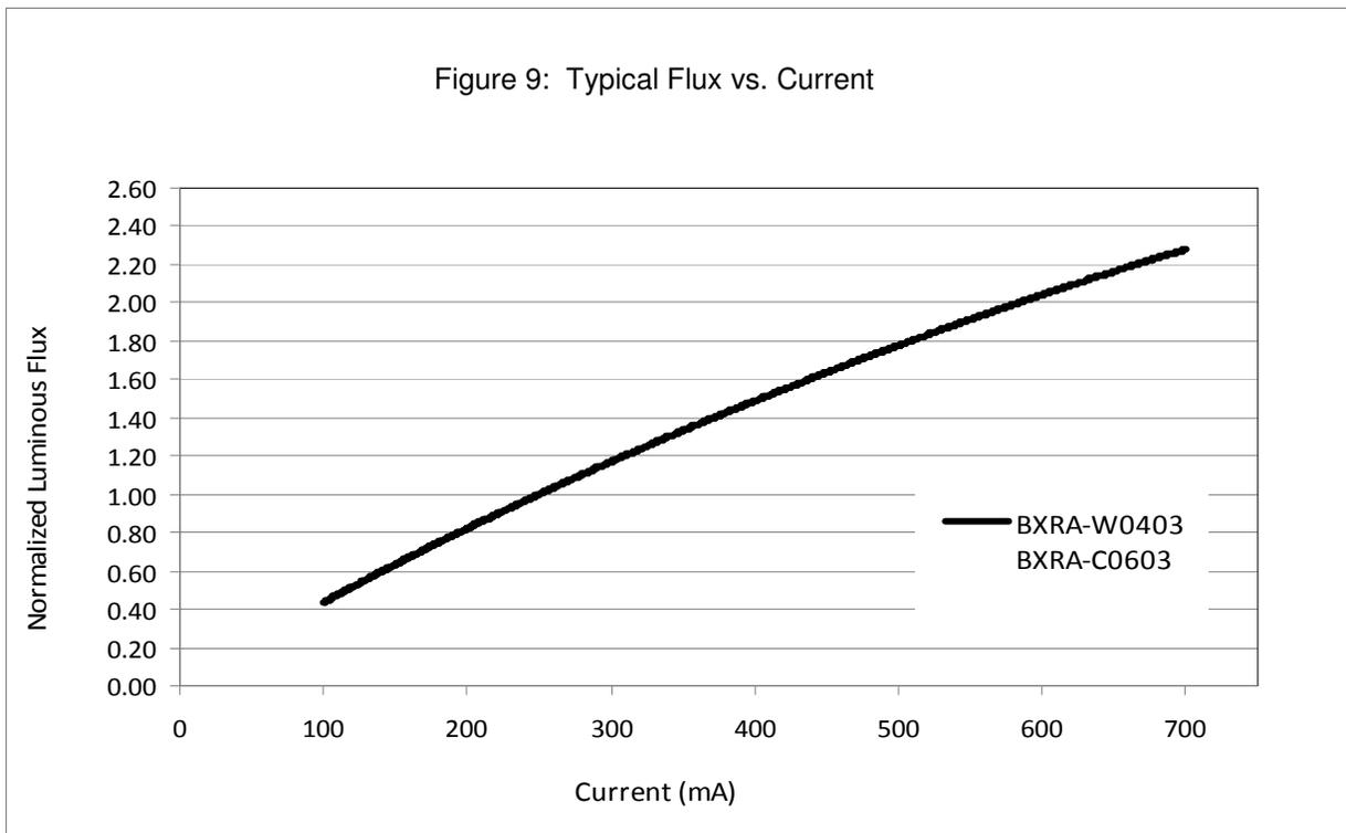
Typical Relative Luminous Flux vs. Current,  $T_j=25^\circ\text{C}$  (continued)
