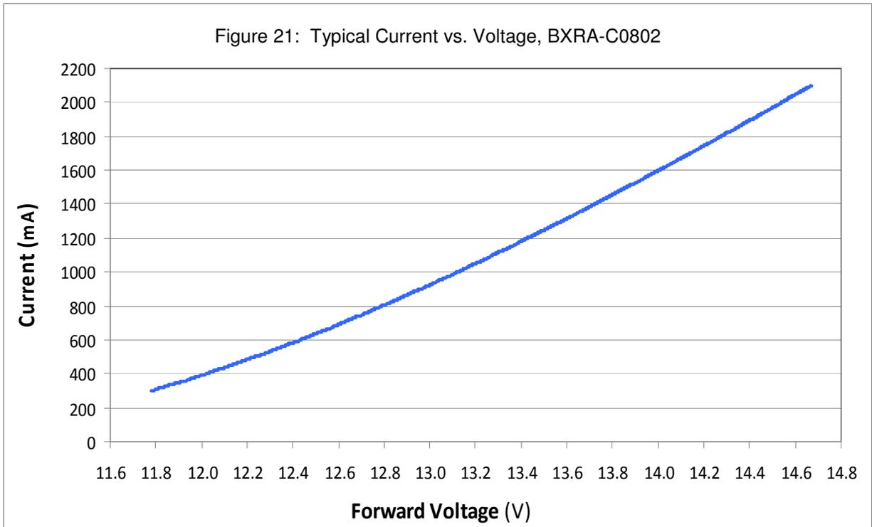
Typical Forward Current Characteristics at  $T_j = 25^\circ\text{C}$  (continued)
