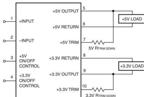
$$5V R_{T_{DOWN}} (k\Omega) = \frac{2.49(V_O - 2.52)}{5 - V_O} - 15 \quad 3.3V R_{T_{DOWN}} (k\Omega) = \frac{2.49(V_O - 1.27)}{3.3 - V_O} - 14.3$$
