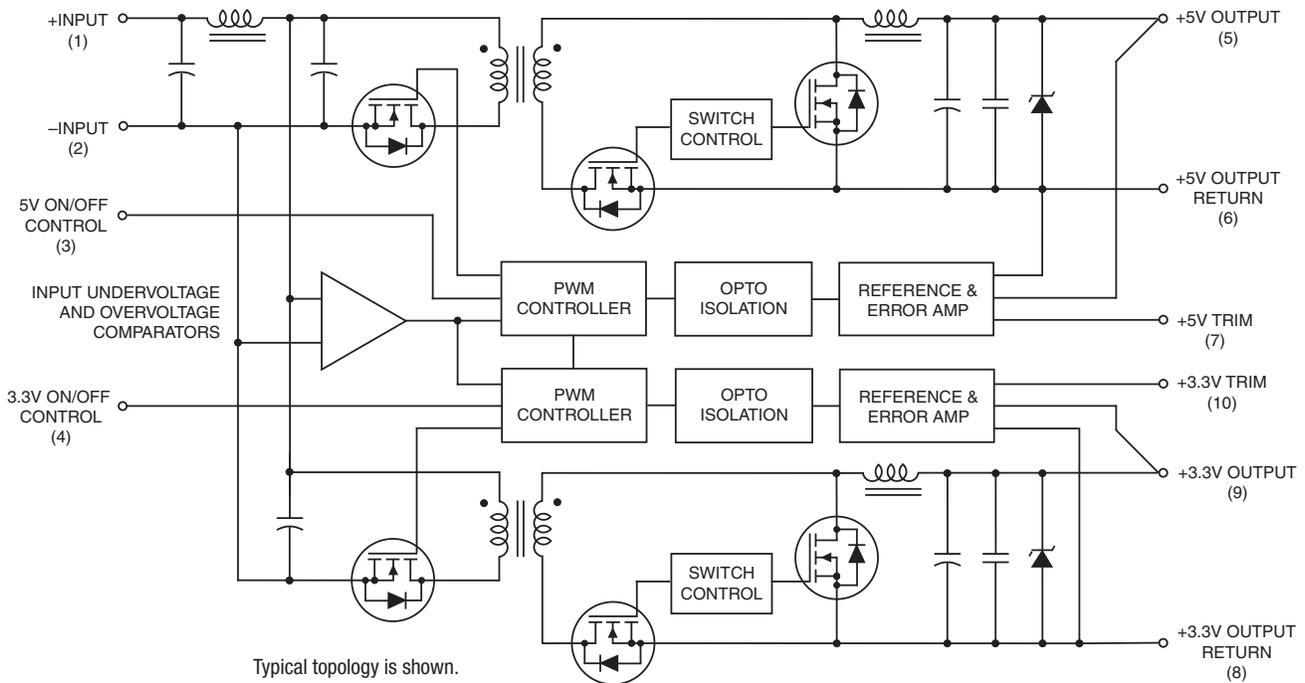
Figure 1. Simplified Schematic
