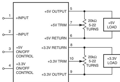
Figure 2. Trim Connections Using A Trim Pot
