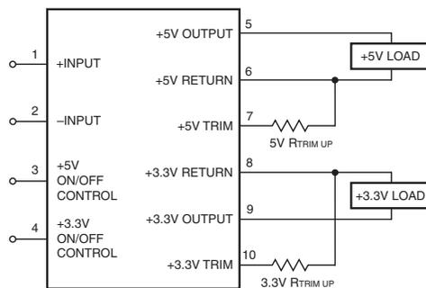
$$5V R_{T_{UP}} (k\Omega) = \frac{6.27}{V_O - 5} - 15 \quad 3.3V R_{T_{UP}} (k\Omega) = \frac{3.16}{V_O - 3.3} - 14.3$$
