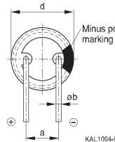
Minus pole The series B41898 has no marking sleeve nor minus pole marking, the positive pole is marked on the aluminum case side instead.
