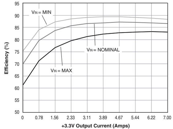
**D12 - 5 Volt Output Efficiency vs. Line and Load (+3.3V @ 700mA)**
