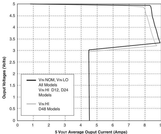
Figure 2b. Current Limiting Characteristics for 5V Output
