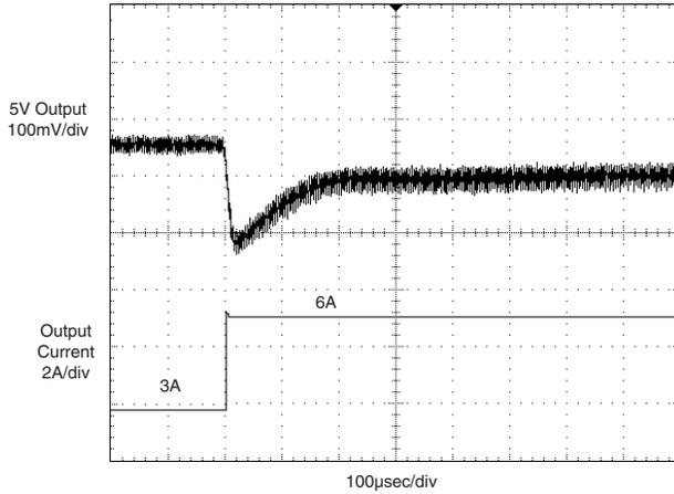
**5V Output Full-Load to Half-Load Transient Response**
