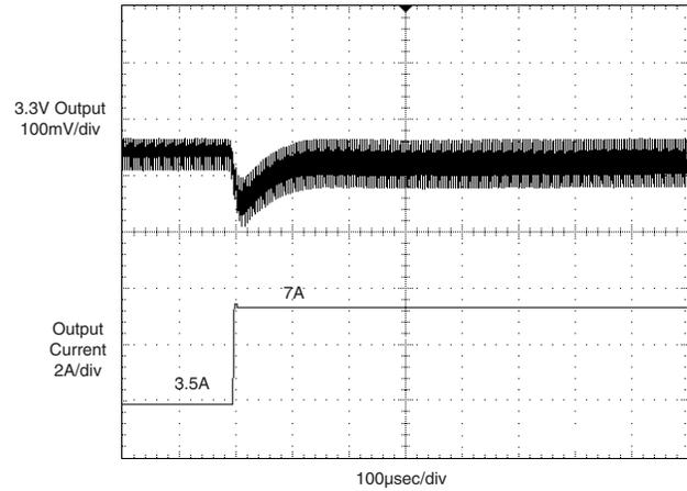
**3.3V Output Full-Load to Half-Load Transient Response**
