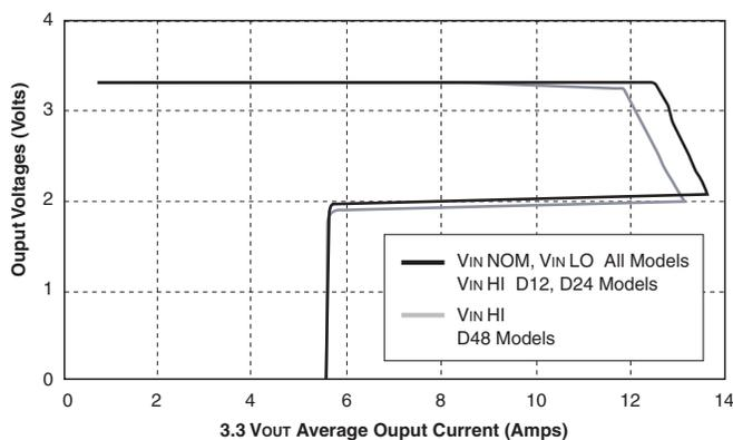
Figure 2a. Current Limiting Characteristics for 3.3V Output
