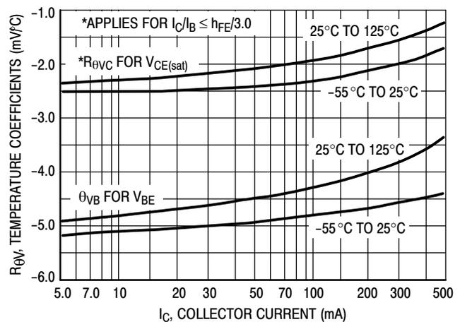
Figure 11. Temperature Coefficients
