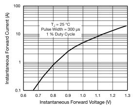
Fig. 4 - Typical Instantaneous Forward Characteristics
