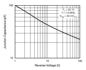
Fig. 5 - Typical Junction Capacitance
