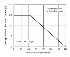
Fig. 1 - Forward Current Derating Curve
