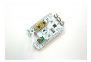
The Ninja Cape features an Atmega328P microcontroller that provides your BeagleBone Black features of Ninja Blocks. This cape is originally manufactured as v1.2 and was modified to be compatible with the BeagleBone Black using the instructions from Ninja Blocks.
