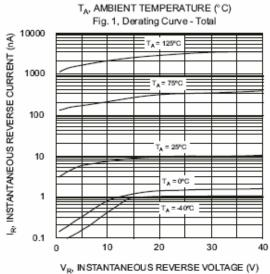
Fig. 3 Typical Reverse Characteristics
