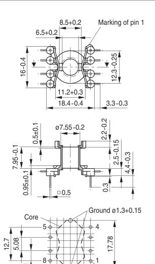
Hole arrangement View in mounting direction
