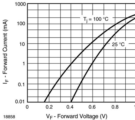
Fig. 1 - Forward Current vs. Forward Voltage
