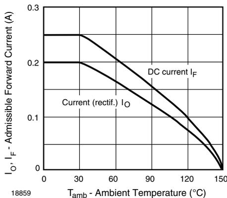
Fig. 2 - Admissible Forward Current vs. Ambient Temperature
