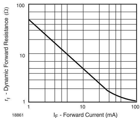
Fig. 4 - Dynamic Forward Resistance vs. Forward Current
