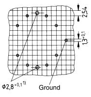
Hole arrangement View in mounting direction
