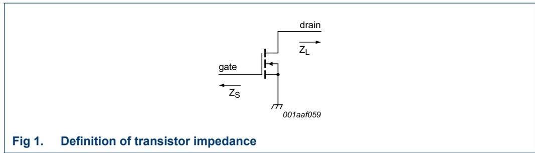
**Fig 1. Definition of transistor impedance**
