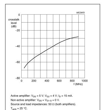
Fig.19 Crosstalk as a function of frequency:
