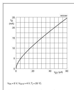
Fig.7 Drain current as a function of gate 1 current; typical values.
