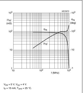
Fig.16 Reverse transfer admittance and phase as a function of frequency; typical values.
