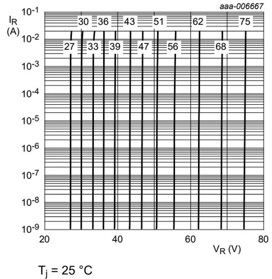
**Fig. 10. Reverse current as a function of reverse voltage; typical values (BZT52H-B/C27 to BZT52H-B/C75)**
