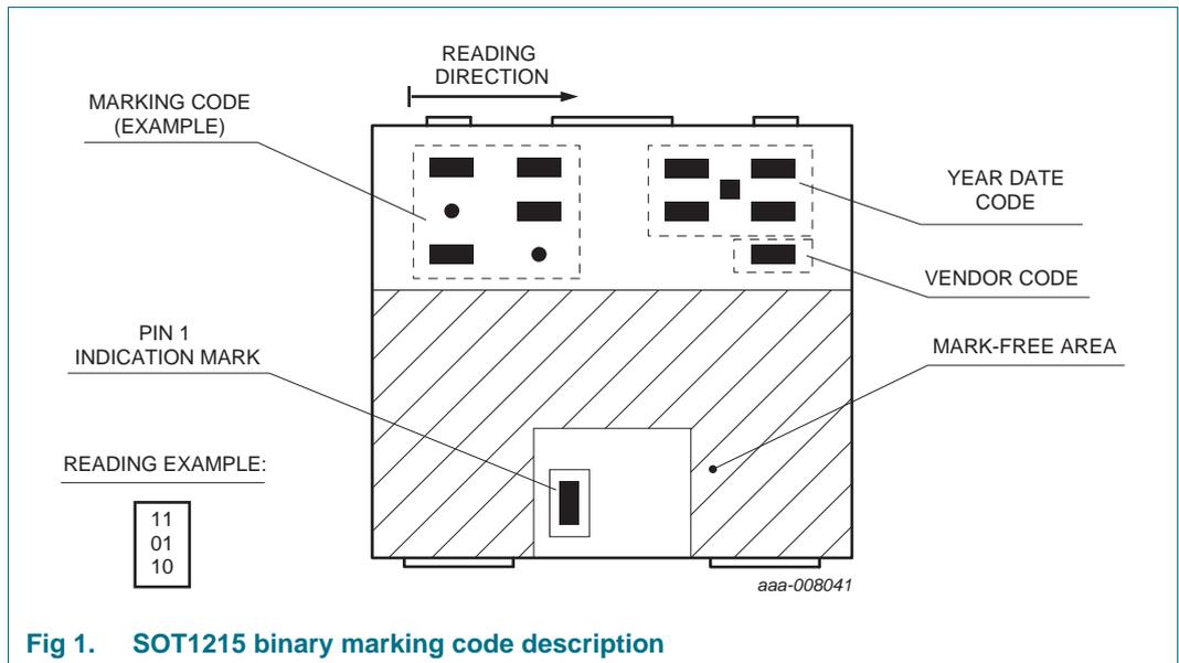
Fig 1. SOT1215 binary marking code description
