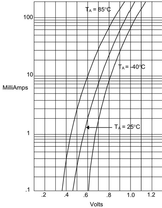
Instantaneous Forward Current - Amperes *versus*
