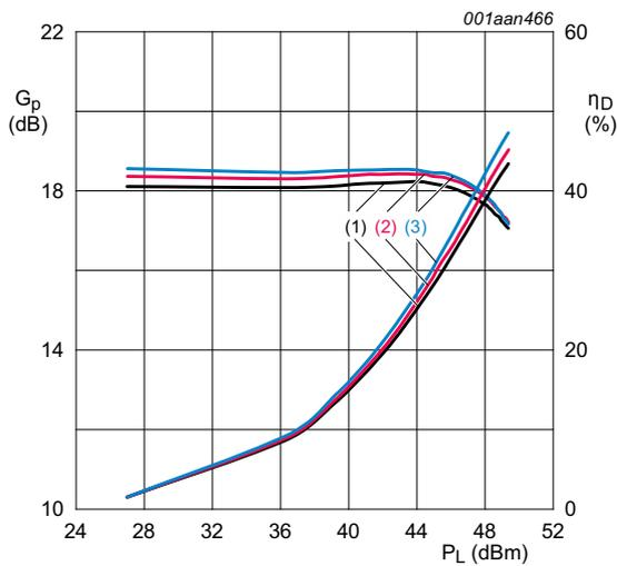
$V_{DS} = 28\text{ V}; I_{Dq} = 1080\text{ mA}$ .
