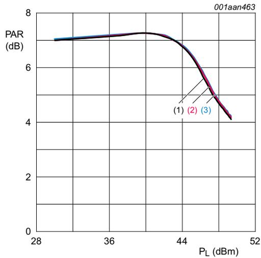
$V_{DS} = 28\text{ V}; I_{Dq} = 1080\text{ mA}$ .
