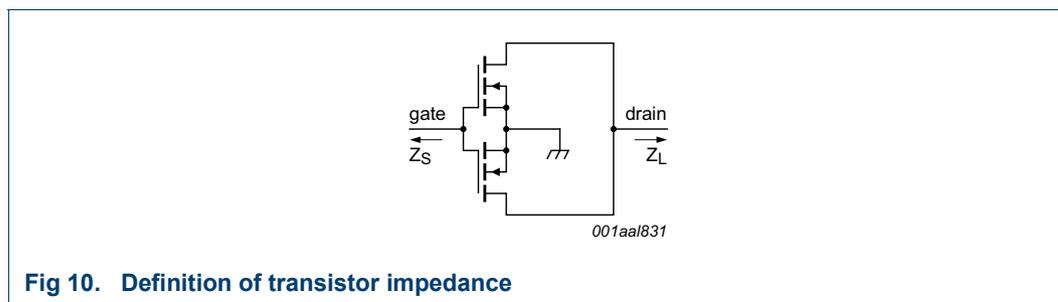
**Fig 10. Definition of transistor impedance**
