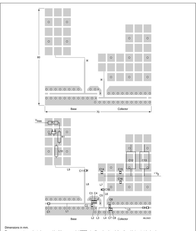
The components are situated on one side of the copper-clad PTFE microfibre-glass board, the other side is not etched and serves as a ground plane. Earth connections from the component side to the ground plane are made by through metallization.
