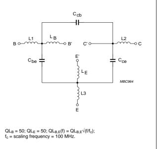
Fig.6 Package equivalent circuit SOT143.
