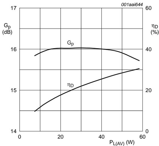
$V_{DS} = 30\text{ V}$ ;  $I_{Dq} = 1400\text{ mA}$ ;  $f = 2140\text{ MHz}$  ( $\pm 5\text{ MHz}$ ); carrier spacing 10 MHz.
