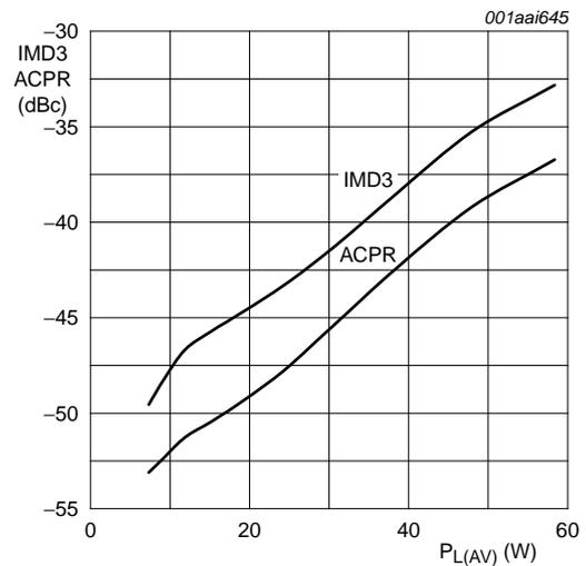
$V_{DS} = 30\text{ V}$ ;  $I_{Dq} = 1400\text{ mA}$ ;  $f = 2140\text{ MHz}$  ( $\pm 5\text{ MHz}$ ); carrier spacing 10 MHz.
