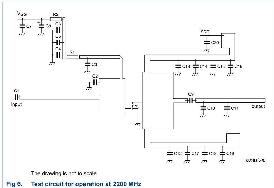
Fig 6. Test circuit for operation at 2200 MHz
