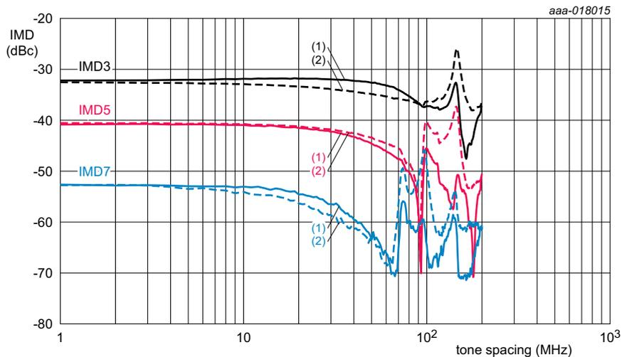
$T_{case} = 25\text{ }^{\circ}\text{C}$ ;  $V_{DS} = 28\text{ V}$ ;  $I_{Dq1} = I_{Dq2} = 100\text{ mA}$  (carrier section, driver and final stages);  $V_{GS1} = 2.55\text{ V}$  (peaking section, driver stage);  $V_{GS2} = 1.47\text{ V}$  (peaking section, final stage).
