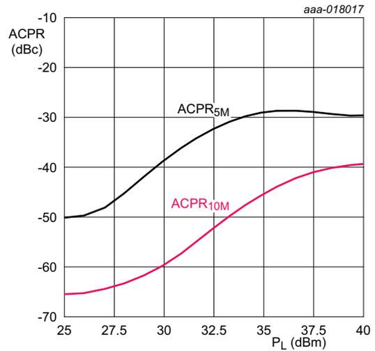
$T_{case} = 25\text{ }^\circ\text{C}$ ;  $V_{DS} = 28\text{ V}$ ;  $I_{Dq1} = I_{Dq2} = 100\text{ mA}$  (carrier section, driver and final stages);
