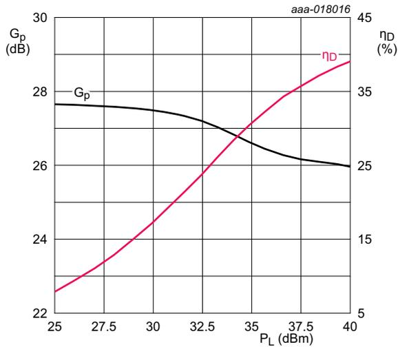
$T_{case} = 25\text{ }^\circ\text{C}$ ;  $V_{DS} = 28\text{ V}$ ;  $I_{Dq1} = I_{Dq2} = 100\text{ mA}$  (carrier section, driver and final stages);
