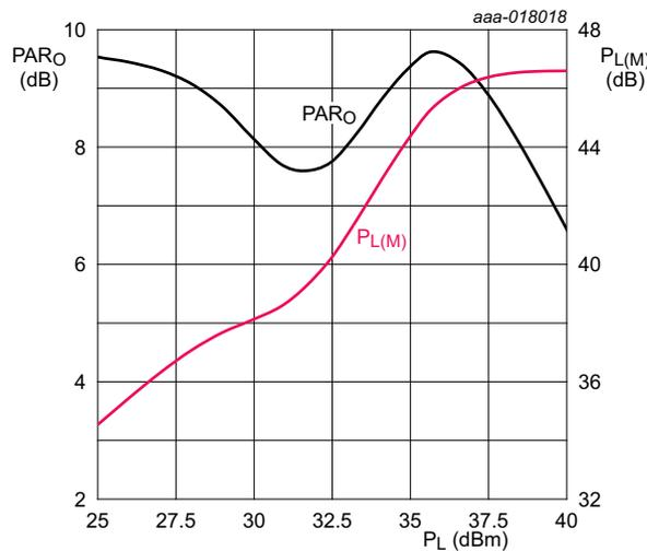
$T_{case} = 25\text{ }^\circ\text{C}$ ;  $V_{DS} = 28\text{ V}$ ;  $I_{Dq1} = I_{Dq2} = 100\text{ mA}$  (carrier section, driver and final stages);  $V_{GS1} = 2.55\text{ V}$  (peaking section, driver stage);  $V_{GS2} = 1.47\text{ V}$  (peaking section, final stage).
