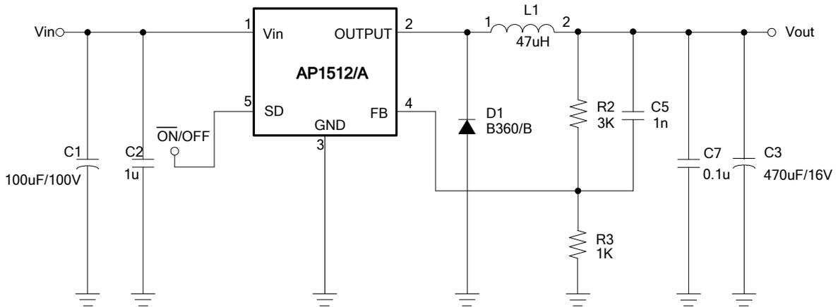
**B.  $V_{in} = 10V\sim 60V$ ,  $V_{out} = 3.3V$ ,  $I_{out} = 0.3A\sim 2A$ ,  $I_{out}$  below 0.3A DCM**
