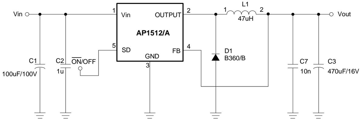
**B.  $V_{in} = 10V\sim 60V$ ,  $V_{out} = 3.3V$ ,  $I_{out} = 0.7A\sim 2A$ ,  $I_{out}$  below 0.7A DCM**
