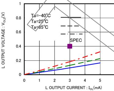
Fig.6 'L' output voltage  $V_{OL2-I_{OL}}$  ( $V_{CC}=2.5V$ )
