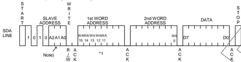
Fig.39 Byte write cycle (BR24G32/64/128/256/512/1M-3A)
