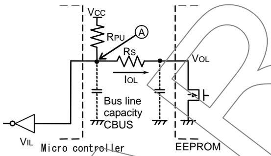
Fig.55 I/O Circuit Diagram
