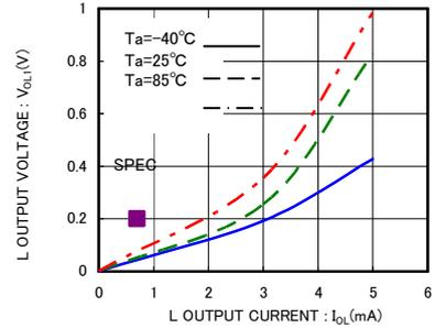
Fig.5 'L' output voltage  $V_{OL1-I_{OL}}$  ( $V_{CC}=1.7V$ )
