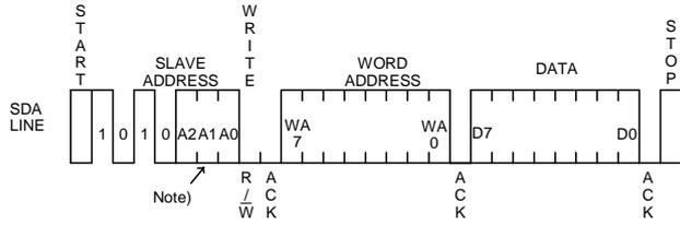
Fig.38 Byte write cycle (BR24G01/02/04/08/16-3A)
