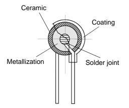
The above picture shows the internal construction of EPCOS ICLs.
