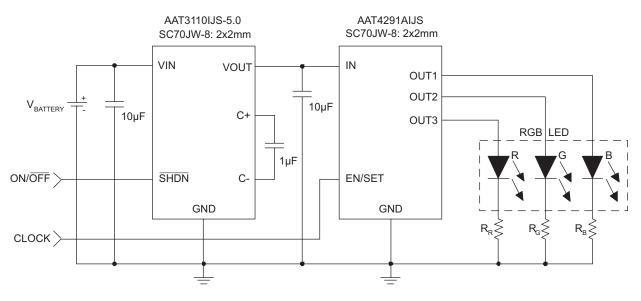
**Figure 2: RGB LED Control** (eliminates three discrete MOSFET switches).
