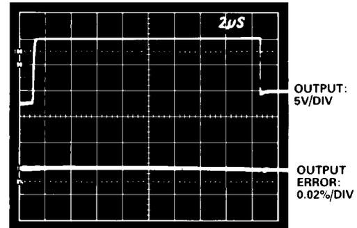
Figure 24. AD840 Settling Demonstrating No Settling Tails
