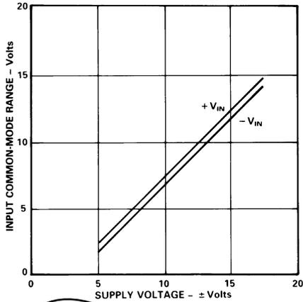
Figure 1. Input Common-Mode Range vs. Supply Voltage
