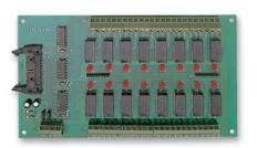
I 6-CH single-pole, double-throw (SPDT form C) relay outputs
