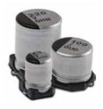
Type AVES Capacitors are rated for 1000 hours at 105 °C with low impedance characteristics. They are ideal for high density PC board packaging. The Type AVES offers a low in-place-cost for a high quality performer. The vertical cylindrical cases facilitate automatic mounting and reflow soldering into the same footprint of like-rated tantalum capacitors except without the need for voltage derating. Type AVES is RoHS compliant.
