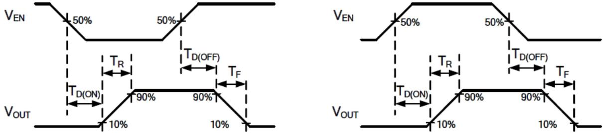
Figure 1 Voltage Waveforms: AP2141D (left), AP2151D (right)
