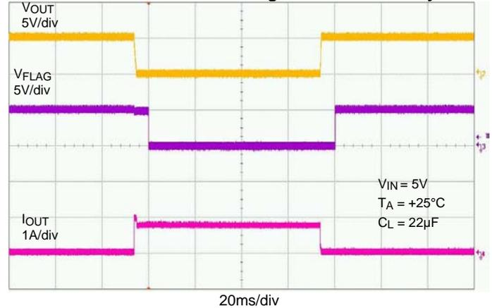
**3Ω Load Connected to Enabled Device**
