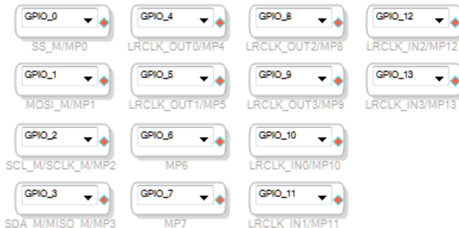
Figure 76. Complete Set of General-Purpose Inputs in SigmaStudio
