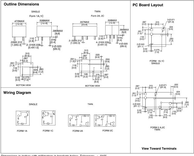
Dimensions in inches with millimeters in brackets below. Tolerance: ± .010"
